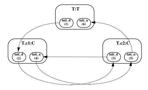
Figure 21—Order of invocation of init\_down and init\_up exec blocks
