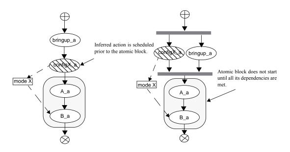
Figure 19—Scheduling graph of atomic block avoiding interference
