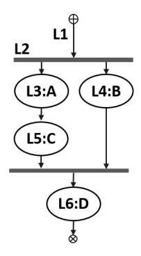
Figure 15—Scheduling graph of join inside sequence block
