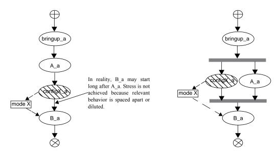
Figure 18—Scheduling graph of action interference
